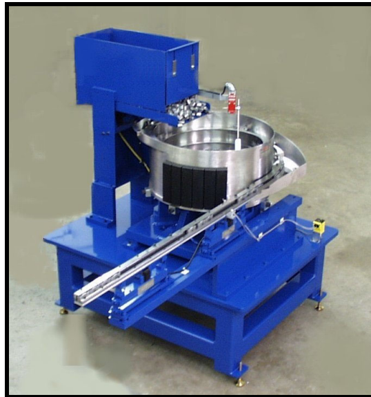
Complete system with a 24" feeder bowl, 36" long inline, table, auxiliary supply hopper, high track shut-off, controllers and a limit switch to control the parts level
