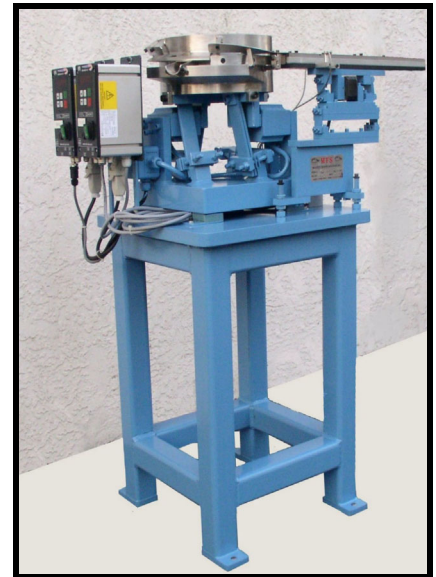
Complete system consisting of a feeder bowl, inline, table and Reo controllers
